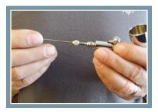
Once the needle is removed, wipe off paint residue with a paper towel. Always wipe the needle from the end to the tip and be careful not to stick yourself, since it is sharp. Once the needle is clean, replace it in the airbrush. Slide it back through the needle chuck screw gently pushing it forward until it stops. Do not push it once it stops. Once the needle is back in place, re-tighten the needle chuck nut.
