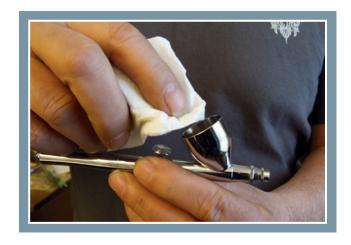
After wiping as clean as possible, squirt airbrush cleaner into the paint reservoir. Spray the cleaner through the airbrush into a rag, paper towel or airbrush spray out pot. Again, wipe the color cup with a paper towel. Use a dental brush to reach into the nooks and crannies of the color cup with the cleaner.
