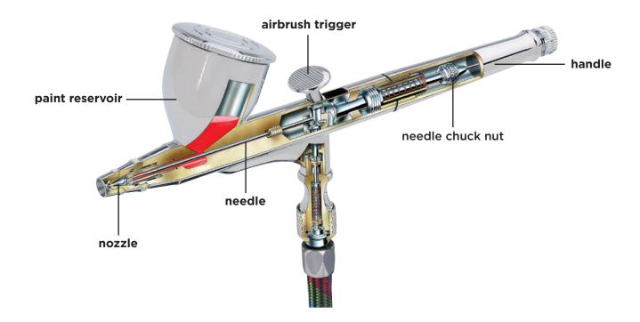
The airbrush requires cleaning only in those areas that come in contact with paint: the paint reservoir or color cup or jar, the tip of the airbrush and the needle. The first thing to do is remove the paint from the paint reservoir. Pour excess paint back into the container and then wipe the reservoir with a piece of paper towel.
