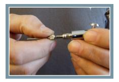
Once the color cup is cleaned, remove the airbrush handle to expose the needle. Notice that there is a nut holding the needle in place. This is called the needle chuck nut and it must be loosened to remove the needle.
